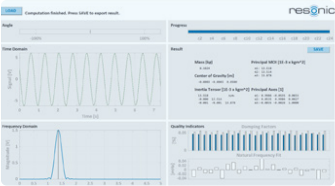
After measuring all 24 positions (in the standard mode), the process is repeated for the empty fixture before the software computes the full mass properties.
